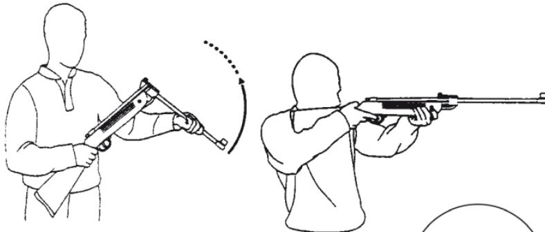
After the pellet has been inserted, close the barrel, it must lock with an audible click. After the safety has been set to "fire", the weapon is ready to fire.
